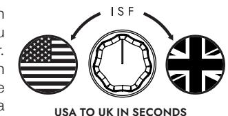
**TIP:** We recommend that to start with the ISF is set to half way and the Bass, Middle and Treble are set to taste. Then try gradually adjusting the ISF CW and CCW until you find the sound you prefer.
